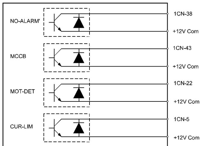
S-Series Servodrive Interlock Interface Output Signals (1CN)
