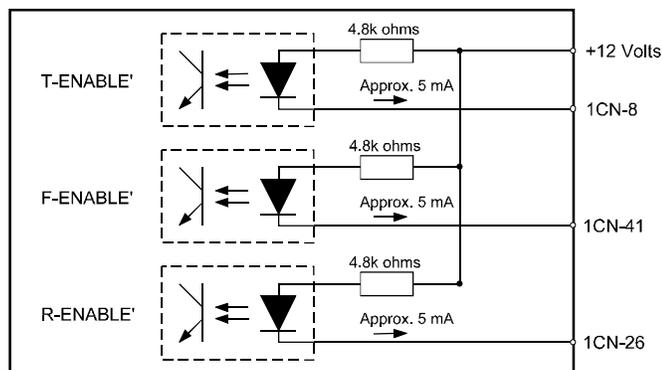
S-Series Servodrive Interlock Interface Input Signals (1CN)
