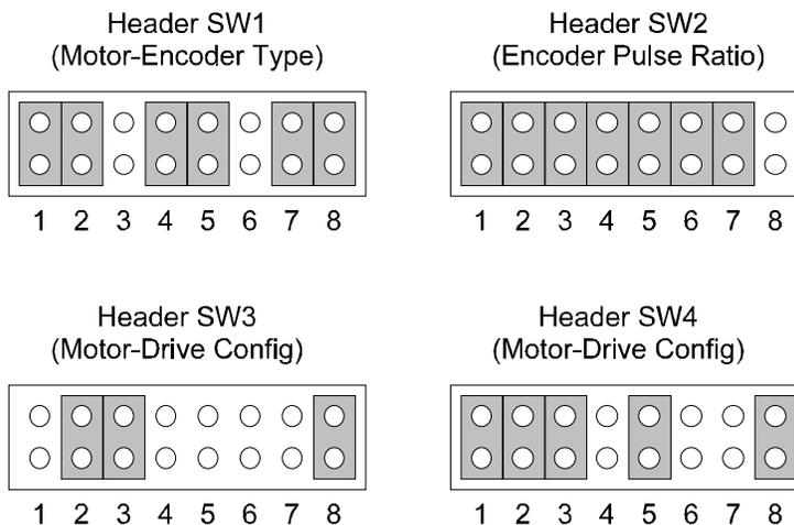
6.2.2.2 Factory Default Jumper Strap Positions for B-Series Motors
