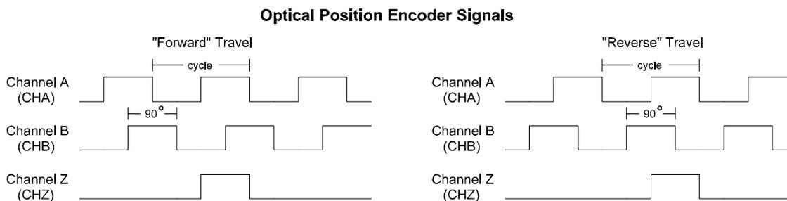
**NOTE:** Channel Z (once per revolution marker channel) is synchronized with Channel A.
