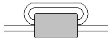
140 Ohm @ 100MHz ferrite core
