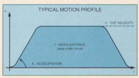
ORMEC motion control technology provides s-curve, linear and parabolic accelerations as standard. For a small non-recurring engineering charge, you can order your own custom acceleration profile.
