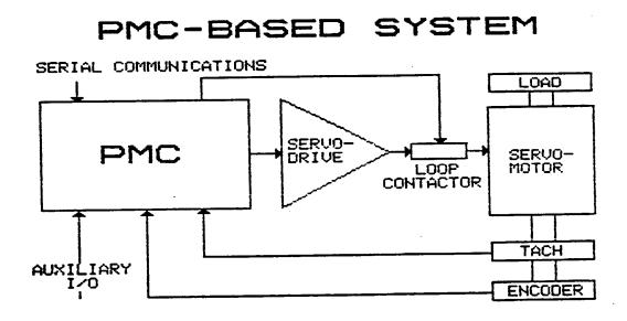
Straightforward, single character, MPL commands may be executed directly from the Serial Communications Interface (SCI), or from non-volatile program memory to create motion control routines. This interactive aspect of MPL greatly reduces the application effort required to implement sophisticated high performance motion control systems compared with alternative approaches.
