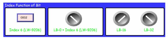
If Index 6 (LW-9206) is set to 2, then switch [LB-0 + Index6] reads LB-32 which is in OFF state.
