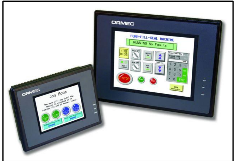
ORMEC's touch screen operator interfaces provide a fully graphical, easy-to-use human-machine interface.
