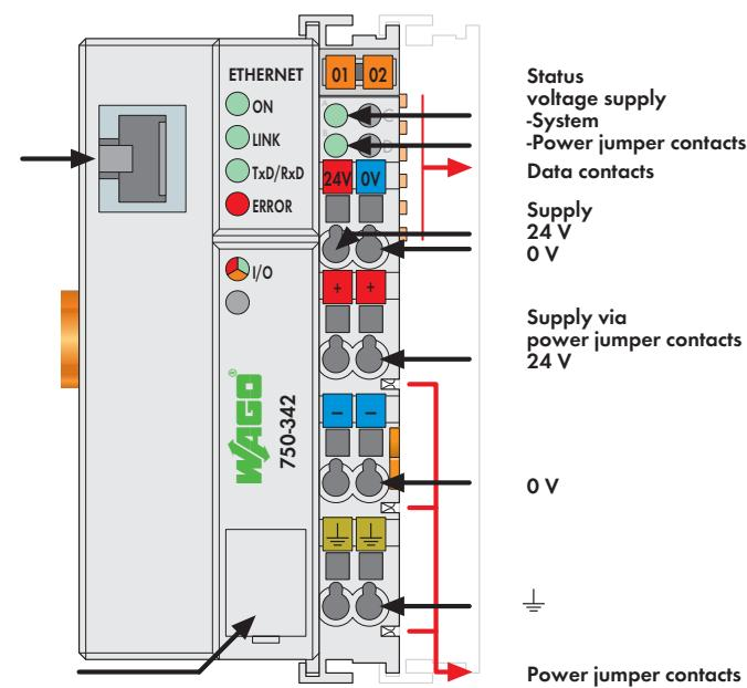
The ETHERNET TCP/IP fieldbus coupler supports a number of network protocols to send process data via ETHERNET TCP/IP. By observing the relevant IT standards, connection to existing local or global networks (LAN, Internet) is possible without any problem.
