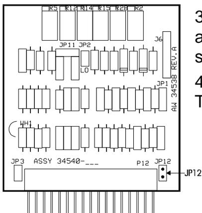
3) If use of the velocity signal developed by the drive and available on J1, pin 3 is not required then remove the shorting plug at JP12.
