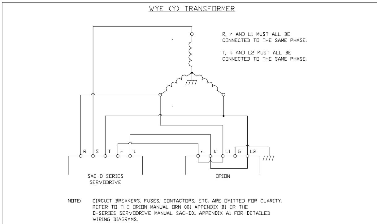
**Figure 1, SAC-D Input Power Wiring for Wye (Y) Transformer**
