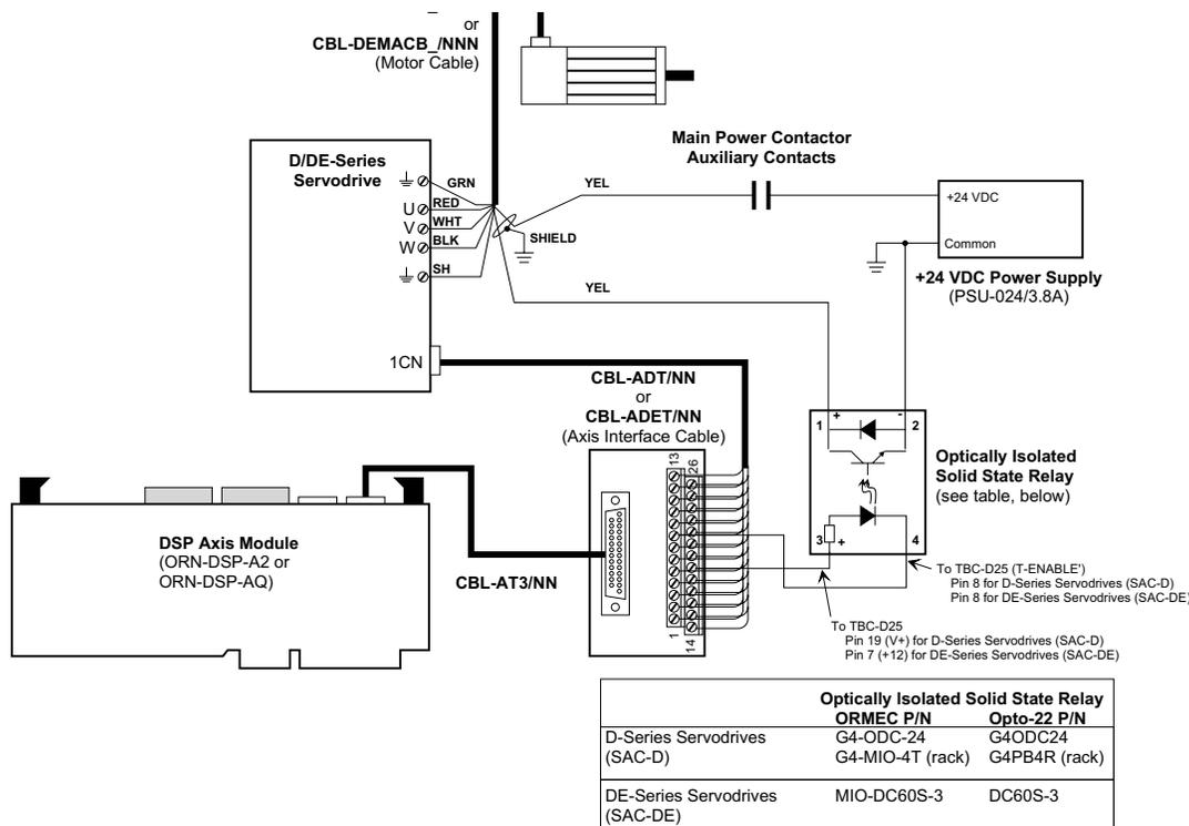
**Figure 4, Fail-Safe Brake Interlock Circuit**
