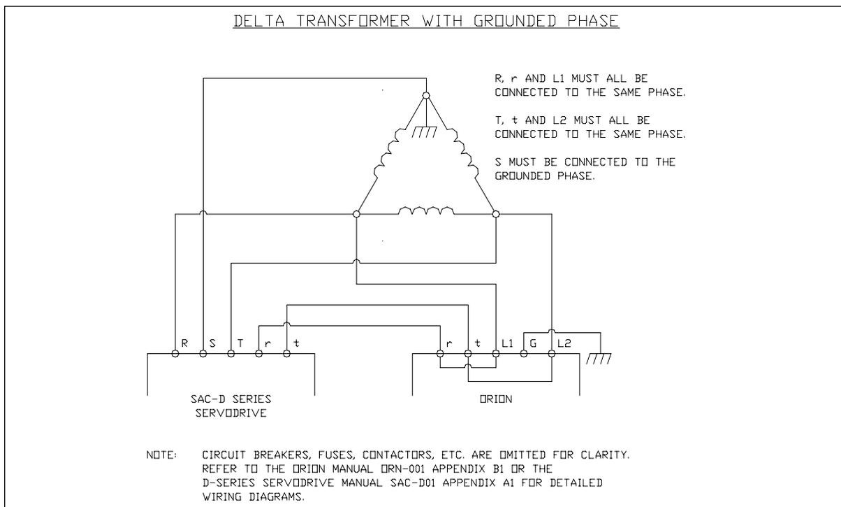
**Figure 2, SAC-D Input Wiring for Delta Transformer with Grounded Phase**
