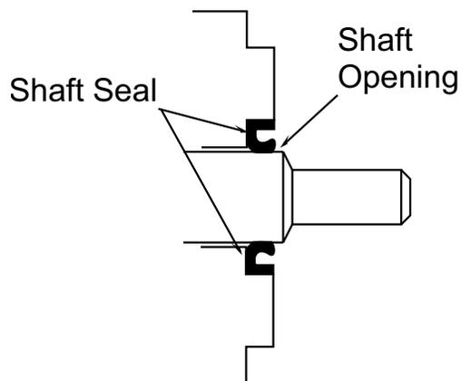
**Figure 13.** Motor Shaft/Oil Seal Cross Section
