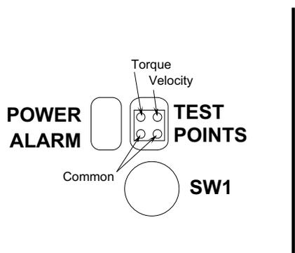
**Figure 11, SAC-D Test Point Layout**
