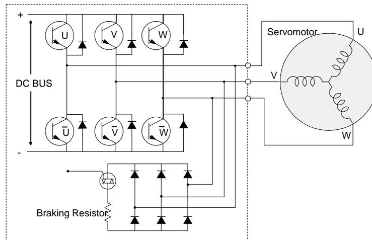
**Figure 7, Dynamic Braking Line Diagram**
