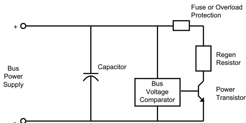
**Figure 6, Shunt Regulator Circuitry**
