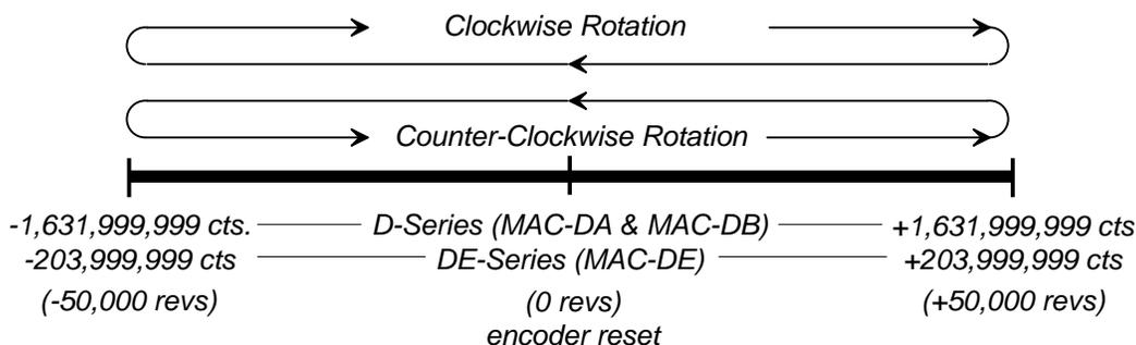
**Figure 9.** Absolute Encoder Wrap-Around
