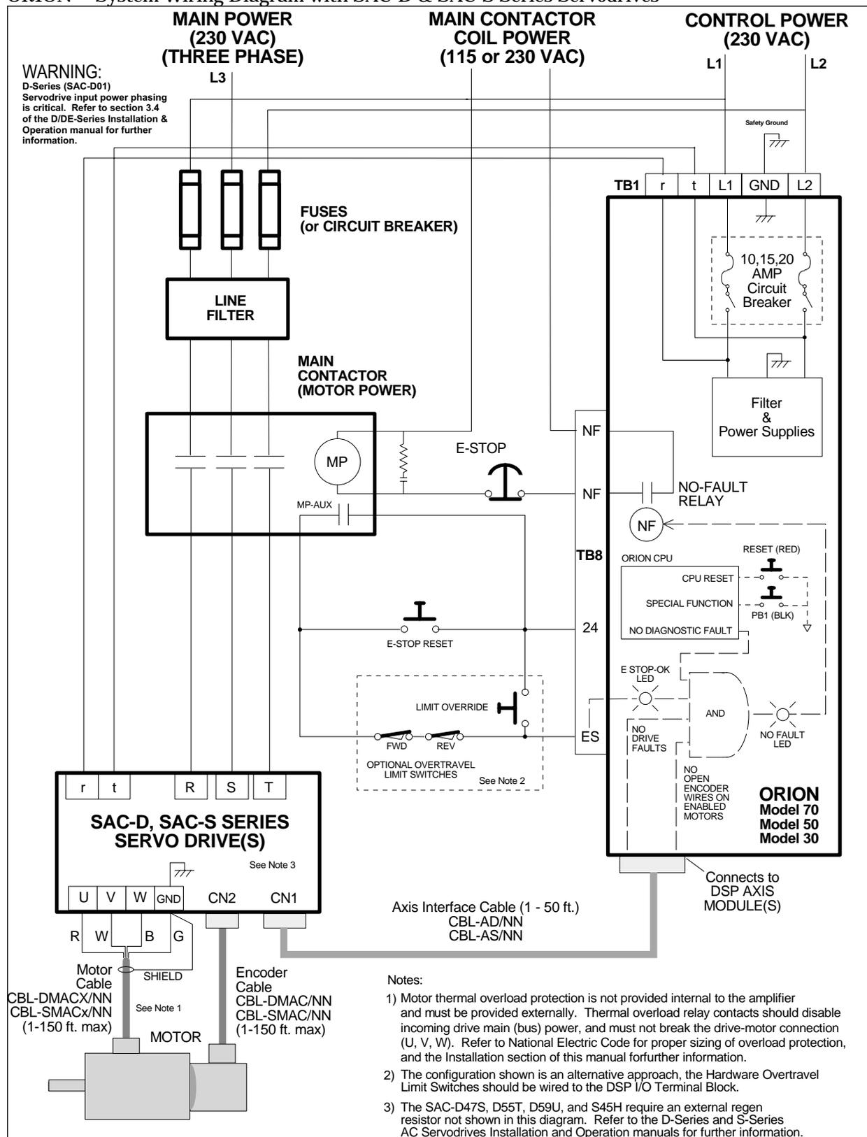
ORION™ System Wiring Diagram with SAC-DE & SAC-E Series Servodrives
