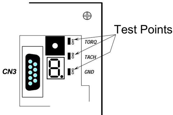
**Figure 12, SAC-DE Test Point Layout**
