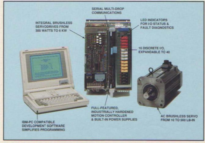
The MCS-S Series offers a plug-together AC brushless motion control system which has the performance needed for the most stringent applications. This highly integrated, modular approach provides a motion system which is cost-effective for single and multi-axis applications. Simply apply power and hook up your motor, and you're ready
