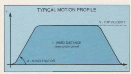
CRMEC motion control technology provides s-curve, linear and parabolic accelerations as standard. For a small non-recurring engineering charge, you can order your own custom acceleration profile.
