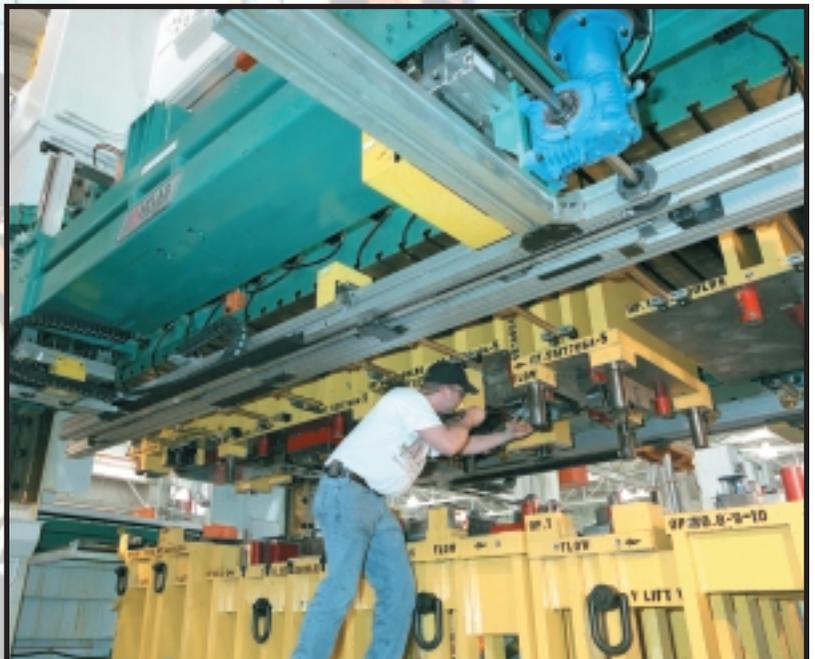
tings that affected the timing of fingers on the in-press transfer system. Coordinating the fingers is critical to lift the parts out of the dies and transfer them forward to the next station.
