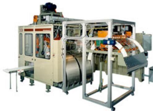
The web is then moved, in most applications, to a separate trim station where the product is trimmed from the web with matched metal punches and dies (some systems used steel-ruled dies for cutting). Once the product is separated from the skeletal web, the scrap is re-granulated and put back into the system.
