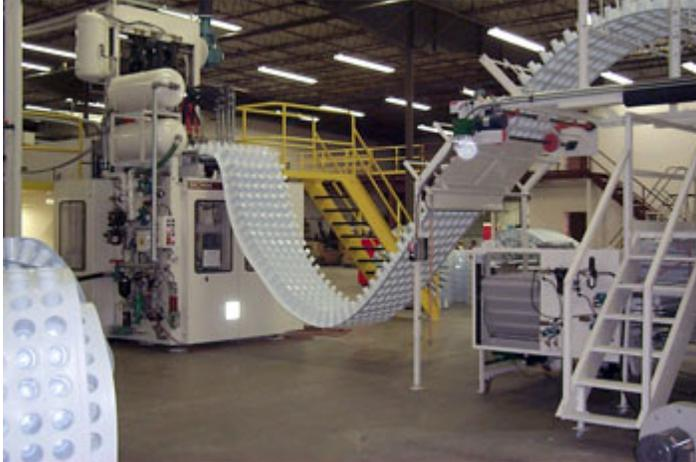
*Servo system on thermoformers uses PLSs to achieve precise multi-axis synchronization, reliability and throughput.*
