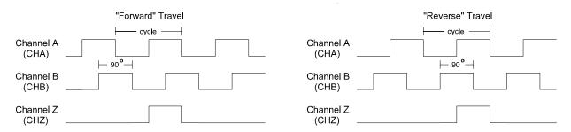
NOTE: Channel Z (once per revolution marker channel) is synchronized with Channel A.
