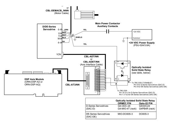
Figure 4, Fail-Safe Brake Interlock Circuit
