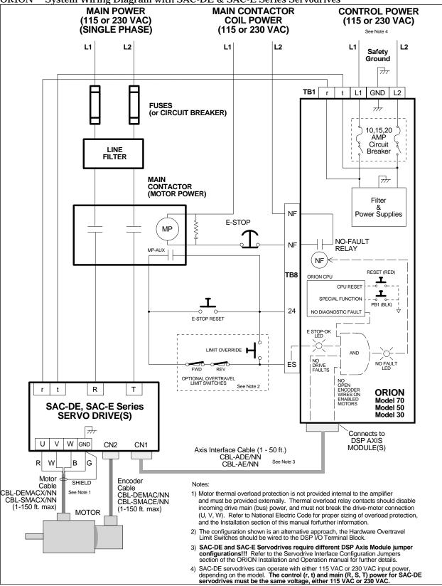
ORION<sup>™</sup> System Wiring Diagram with SAC-DE & SAC-E Series Servodrives
