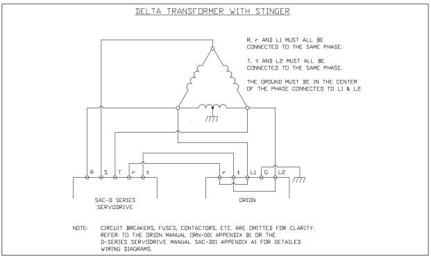
Figure 3, SAC-D Input Wiring for Delta Transformer with Stinger
