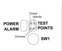
Figure 11, SAC-D Test Point Layout
