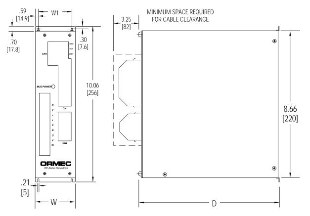
MINIMUM VENTILATION CLEARANCE: 2" [50 MM] ABOVE AND BELOW, AND 0.6" [15 MM] BETWEEN SERVODRIVES.
