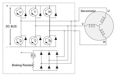
Figure 7, Dynamic Braking Line Diagram
