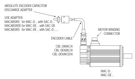
Figure 8, Absolute encoder reset adapter
