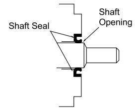
Figure 13, Motor Shaft/Oil Seal Cross Section
