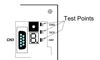
Figure 12, SAC-DE Test Point Layout
