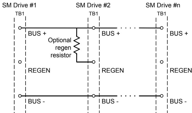
**Figure 15, Bus Sharing Connections**
