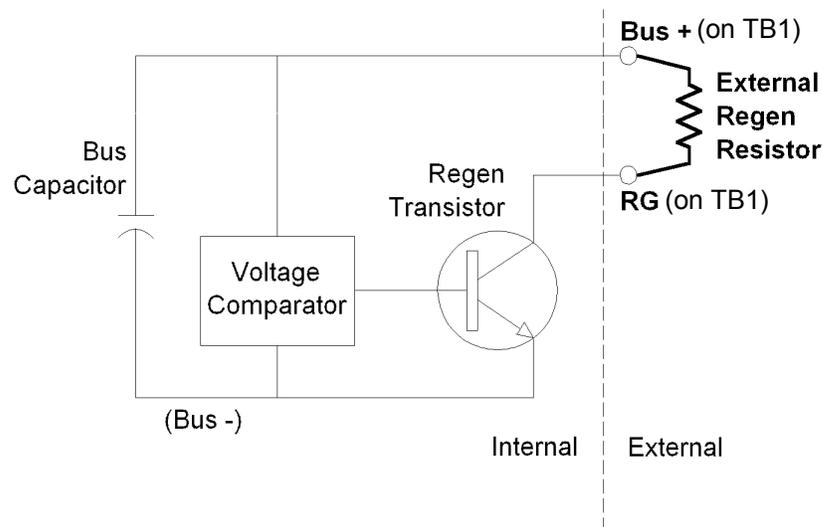
**Figure 14, Regen Resistor Connection**
