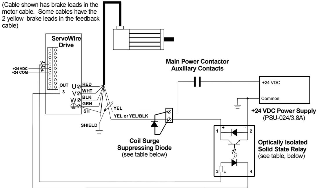
**Figure 19**, Fail-Safe Brake Interlock Circuit
