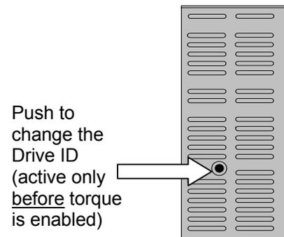
Figure 17, Top View of ServoWire SM Drive showing Drive ID Pushbutton
