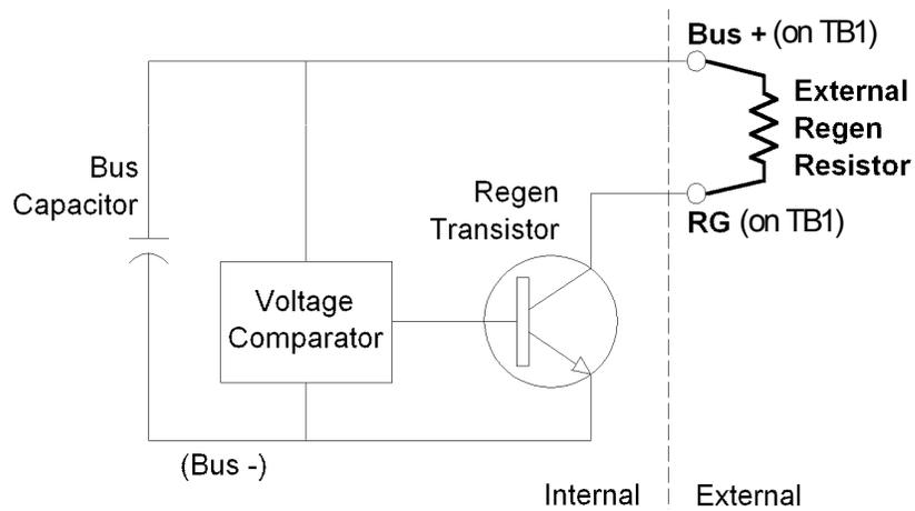
Figure 26, Simplified Schematic of Shunt Regulator
