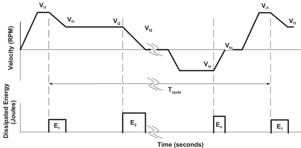
Figure 27, Regeneration during deceleration.
