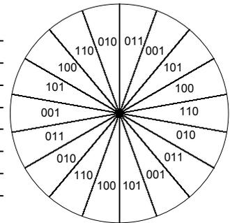
Figure 24, Valid Hall States (6 Pole Motor Example diagram)
