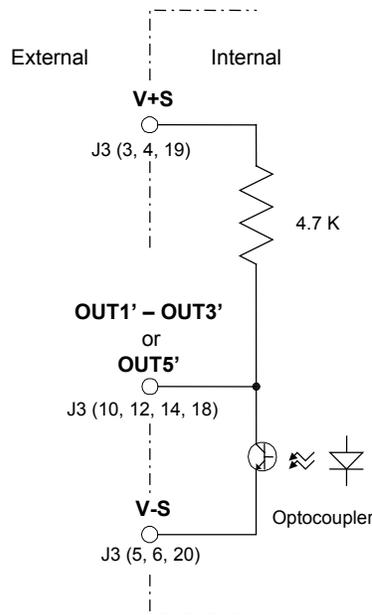
**Figure 13, Schematic of Discrete Outputs OUT1'-OUT5'**
