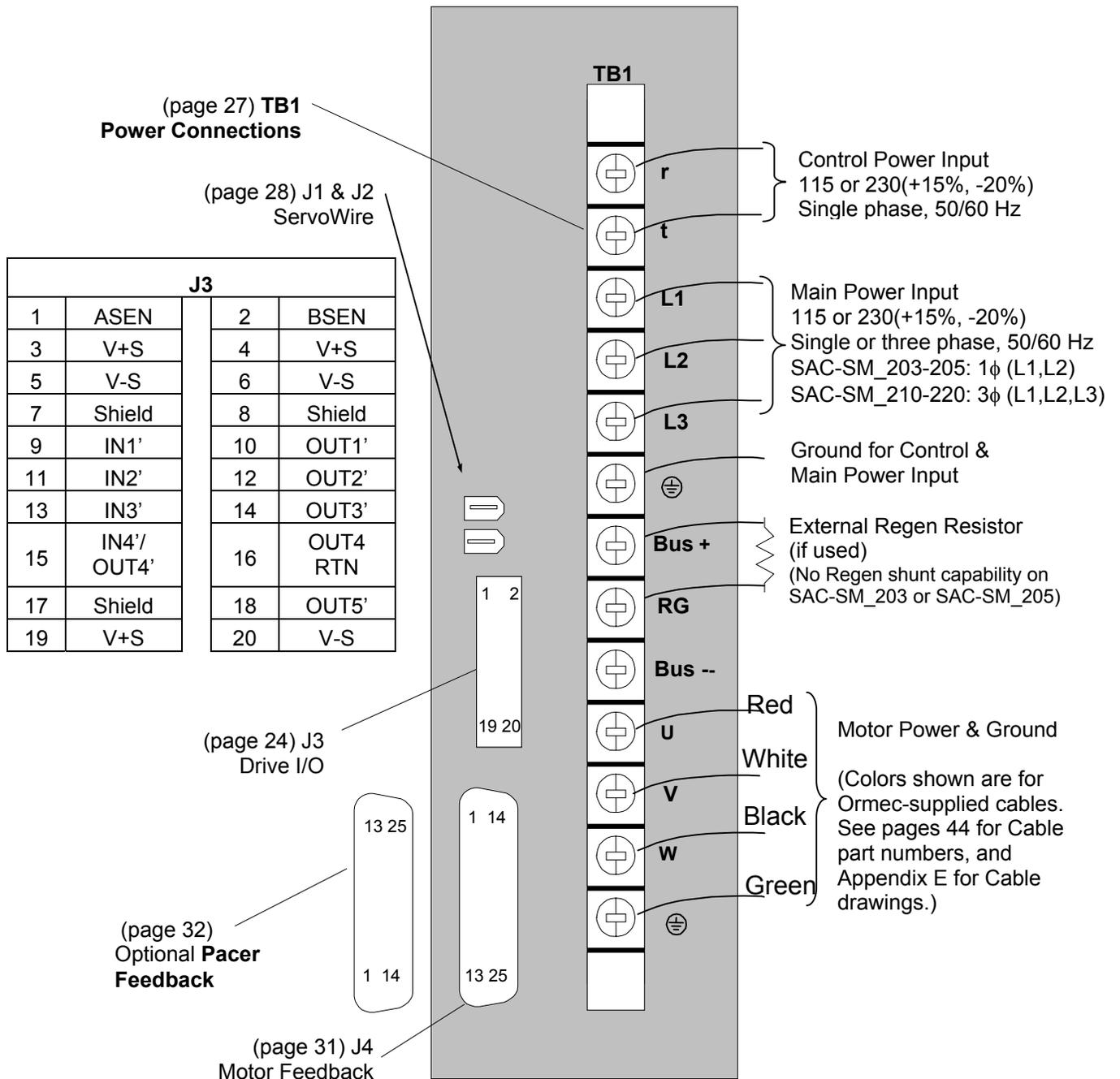
**Figure 6, ServoWire SM Drive Connections Overview (SM\_203 – SM\_220)**
