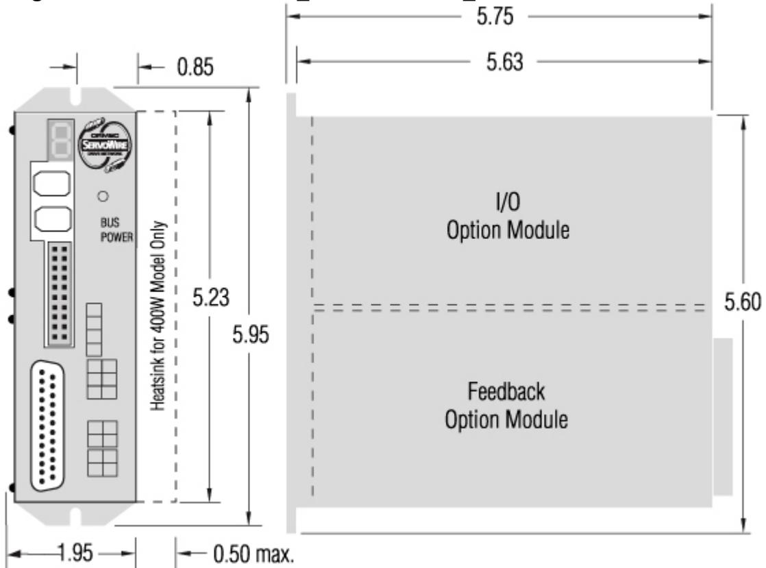
Additional clearance above, below and to the sides of the ServoWire Drives is also required for heat dissipation:
