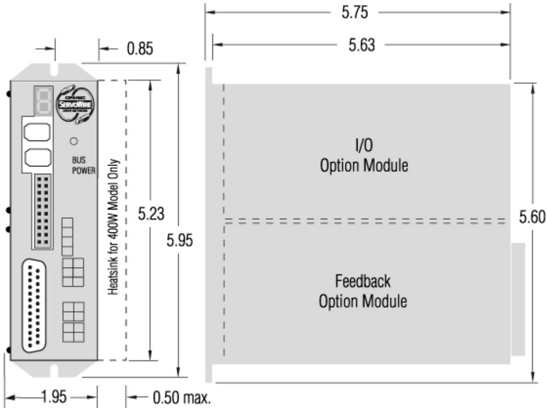
**Figure 4, ServoWire SM Low Power Drives (24-96 VDC) Outline Drawing**
