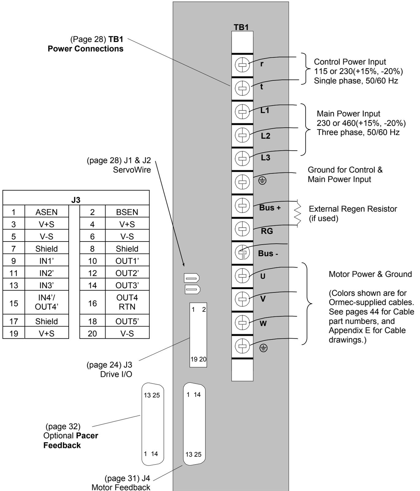
Figure 8, ServoWire SM Drive Connections Overview (SM\_405 – SM\_410)
