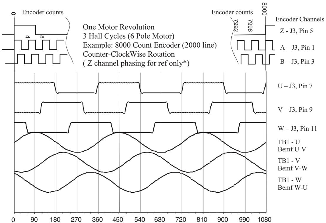
Figure 23, Hall signals and Motor Back EMF waveforms
