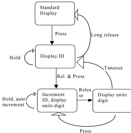
Figure 16, Drive ID Setup Flowchart
