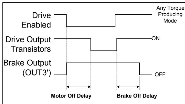
**Figure 21**, Brake Output Sequence of Operation
