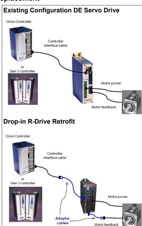
The R-Drive efficiently replaces existing ORMEC SAC-DE Series Servo Drives for ORION and GEN 3 controller applications.
