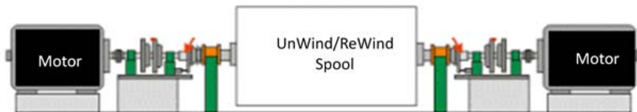
Figure 2: UnWind/ReWind Section of a large spool controlled by two servo motors.
