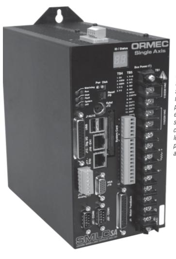
The ServoWire Motion & Logic Controller -Single Axis (SMLC-SA) is a standard offthe-shelf, cost-effective control platform. Program motion control and logic using standard IEC 61131-3 tools. PLCopen standard motion control function blocks plus powerful ORMEC extensions reduce your software development costs and bring new levels of motion performance to singleaxis applications.
