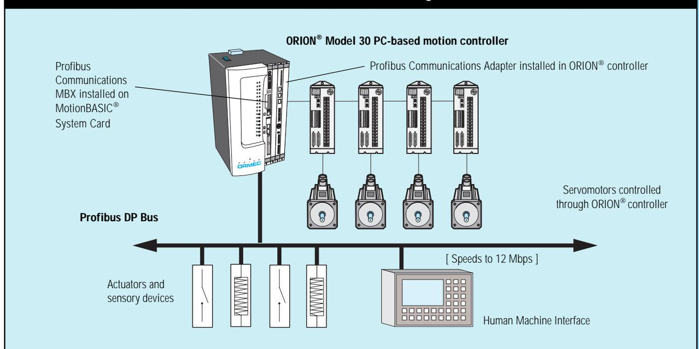
High-speed, time-critical data transmission at the fieldbus level is defined by the Profibus DP specification.
